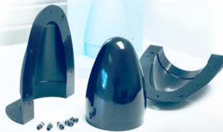
VARTM tooling with autoclaved rocket nosecone fairing
